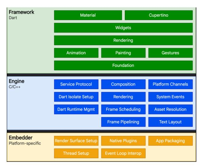
To the underlying operating system, Flutter applications are packaged in the same way as any other native application. A platform-specific embedder provides an entrypoint; coordinates with the underlying operating system for access to services like rendering surfaces, accessibility, and input; and manages the message event loop. The embedder is written in a language that
